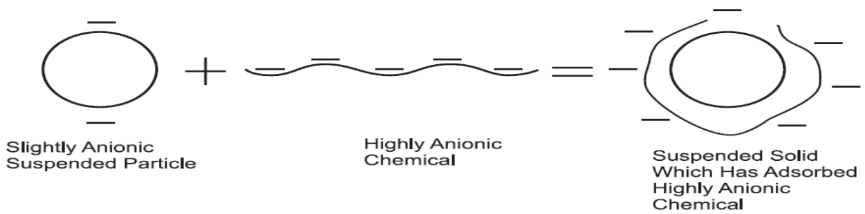
FIGURE 19.4 Suspended particle adsorbs highly anionic polymer, greatly increasing surface charge.
