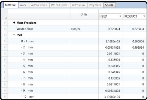
11. Repeat the same task of reducing the particle size of "FEED" stream but this time using the third method, that is, "Specify outlet PSD" (see Figure 14.9). Under "Specifications" tab, select "Substream ID" as CIPSD; select "Use distribution function"; the "Bypass fraction" is set to 0; create a new distribution function ID and nameit 1; select the "Distribution function" as Normal; select D50 parameter with 1mm and standard deviation of 1 mm.
