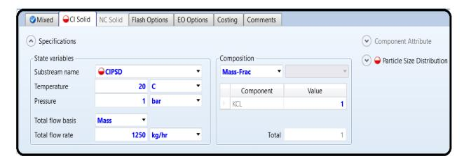
Notice that the half-filled red circle shown in Figure 14.3 indicates that input data pertaining to "FEED" stream is still incomplete, and the reason for this is simply because the stream class is of "MIXCIPSD" type with a substream of "CIPSD" type. Under such stream and substream definitions, we need to define or associate a PSD with the feed stream as well as define a simulation PSD for presentation of results.
