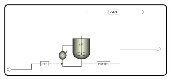
5. Figure 14.29 shows the feed stream properties in terms of *P*, *T*, and compositional flowrate. There will be no need for PSD specification because the feed stream is a saturated aqueous KCl solution entering at the maximum solubility, which is 35 g KCl/100 g water (amounts to KCl mass fraction of 0.26).
